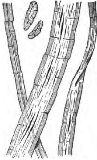
FIG. 4. — Ramie. (After Hassack.) 200 Diameters.
